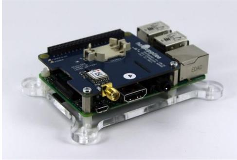
Attach the larger stand offs to the perspex case using supplied metal screws.
