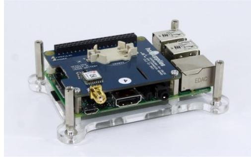
Finally attached the top perspex case with the supplied metal screws :
