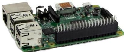
Screw two of the small nylon stand offs supplied with the Geaux Robot case through the two mounting holes next to the header on the Pi. Use the supplied nylon screws to secure.
